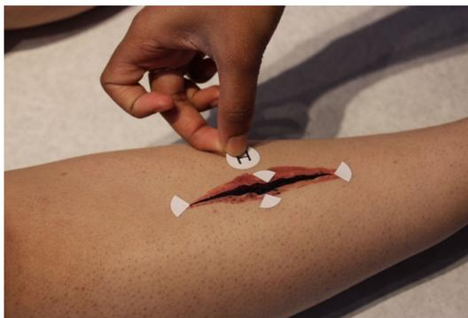
**FIGURE 2:** An example of a two-dimensional tattoo applied to the participant's skin, along with four three-dimensional markers surrounding it. Three-dimensional markers were necessary for making reference measurements with the FARO Edge ScanArm, as it does not detect color.
