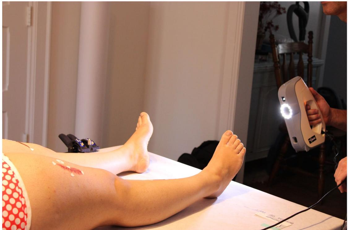
**FIGURE 1:** An Artec Eva being used to scan a live participant.
