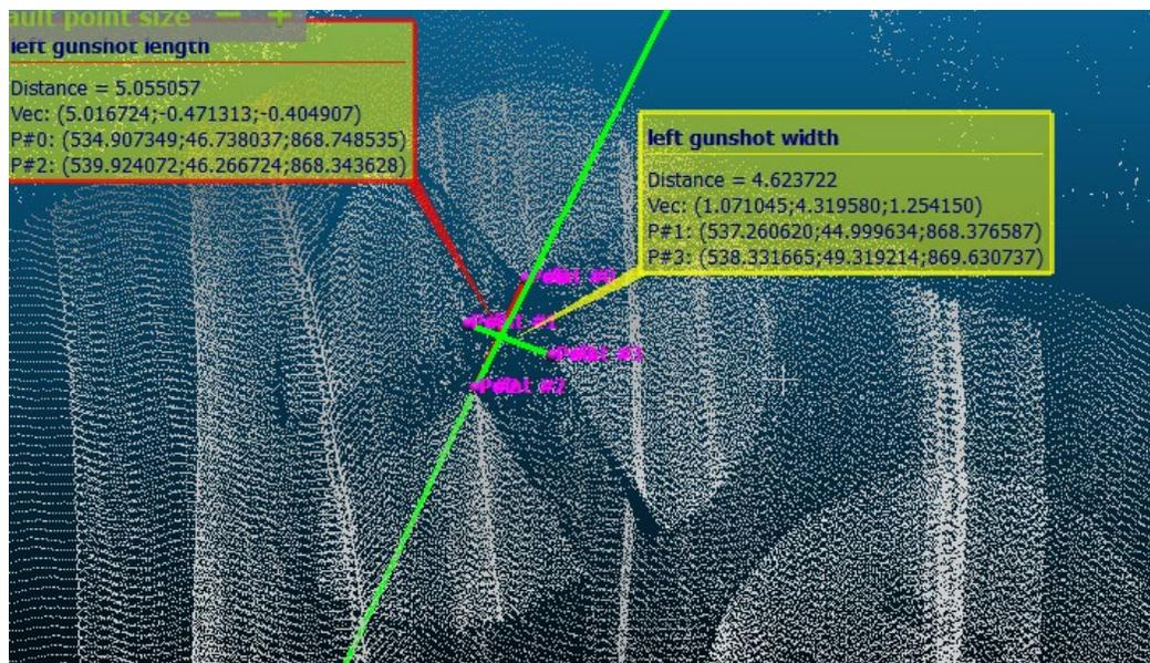
**FIGURE 4:** An example measurements taken on a tattoo in CloudCompare v2.6.0. The purple dots represent points manually picked to define the distance being measured. The four three-dimensional markers can be seen surrounding the tattoo, and the tips of the markers allowed for accurate point picking.
